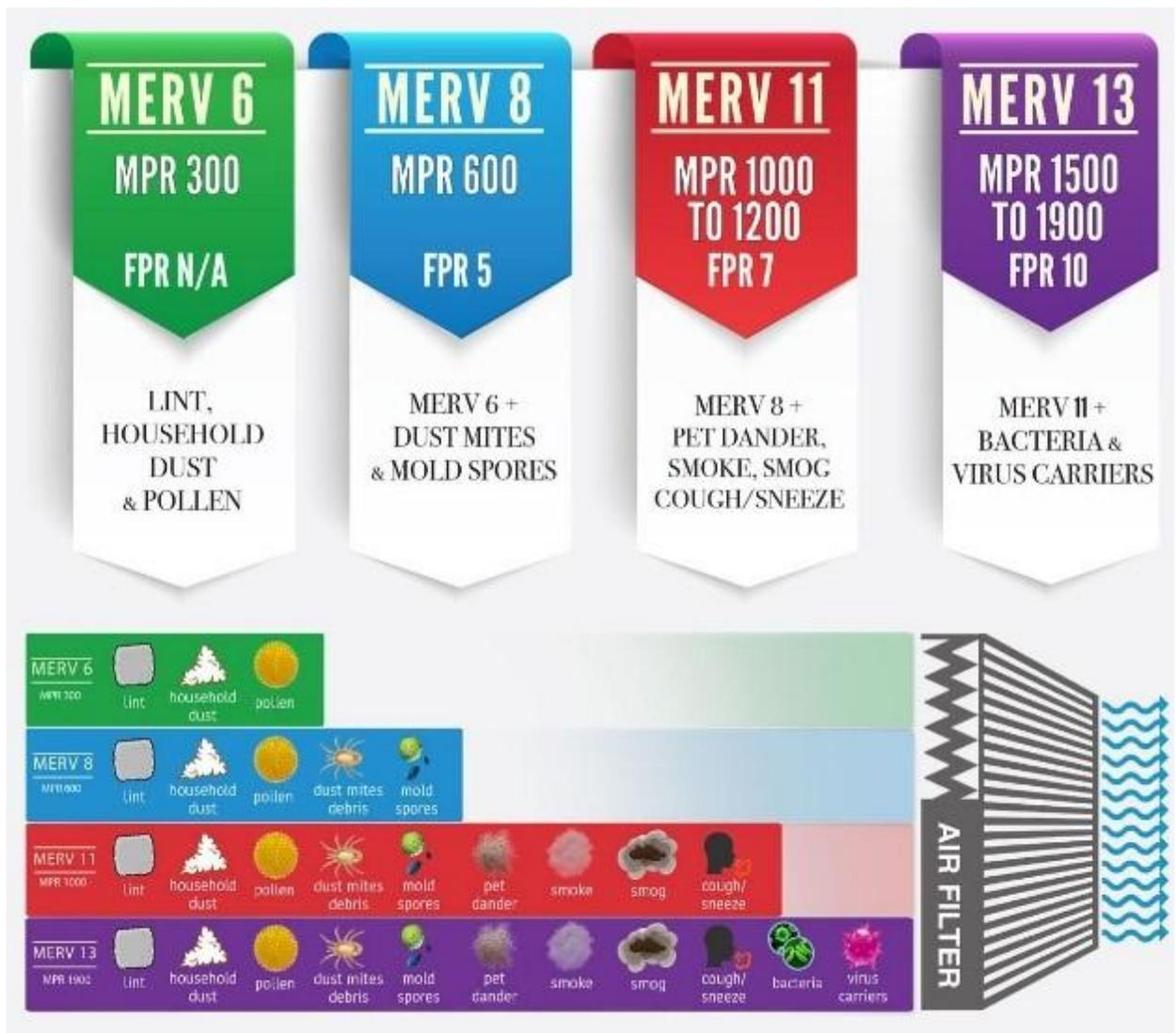
Use of a filter to this higher standard provides the initial service of maximum filtering of the air entering the sanitizing chamber of our unit system. This ultra fine screening also serves to trap or slow sub micro organisms (such as some viruses and bacteria) that are less than .3 microns will be able to pass through however, the movements of navigating through the filter tends to slow the particle within the suspension of the air flow. This is crucial to our next step in air cleaning.
